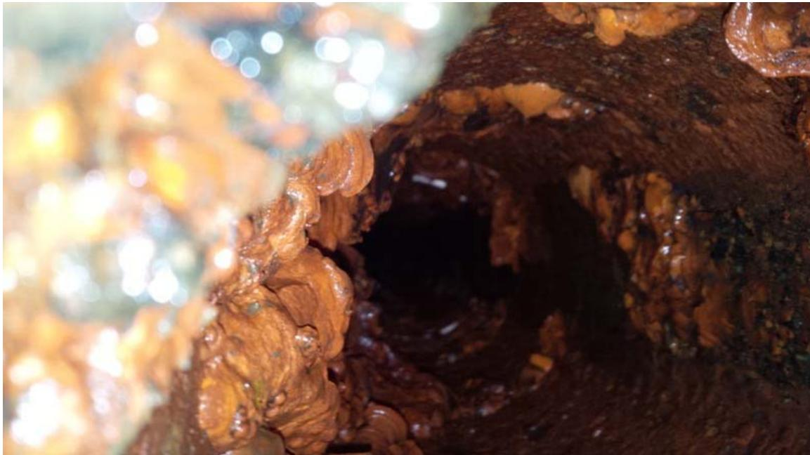
*Figure: Tuberculated cast iron pipe found on Main Street in Glencoe*
