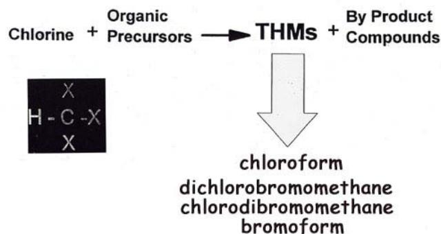
Figure: Basic diagram representing the formation of THMs
