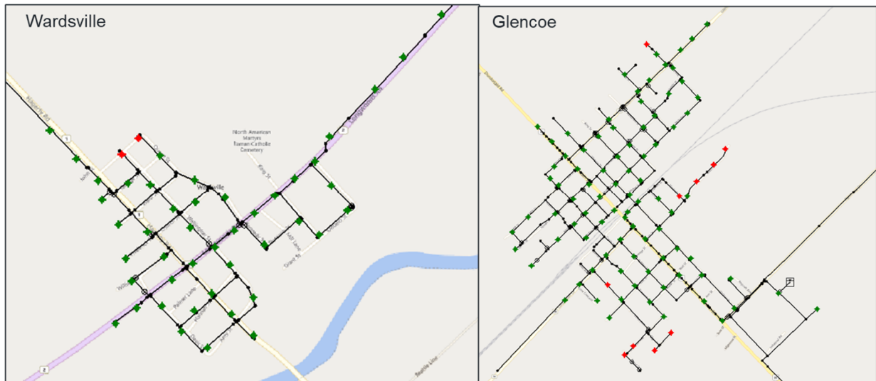
Figure 11: Simulated Fire Flow Lower than 50 L/s in Wardsville and Glencoe under 2041 MDD
